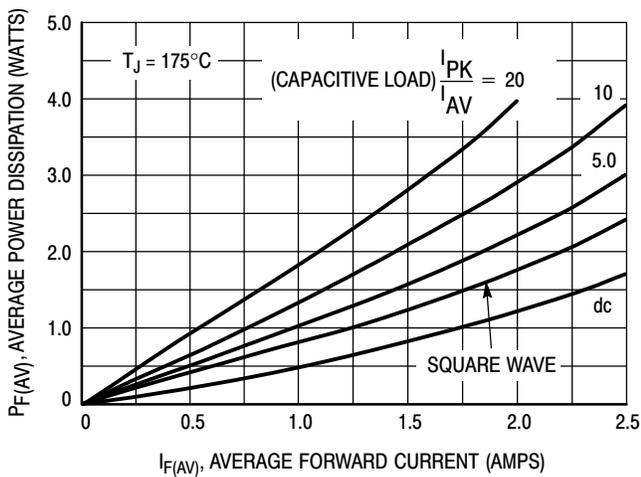
**Figure 4. Power Dissipation**
