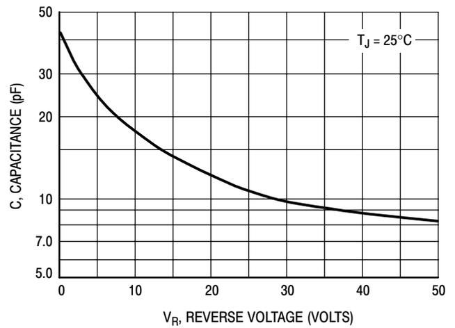
**Figure 5. Typical Capacitance**
