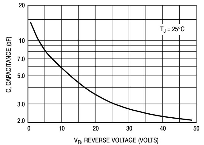
**Figure 10. Typical Capacitance**
