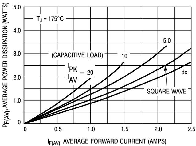
**Figure 9. Power Dissipation**
