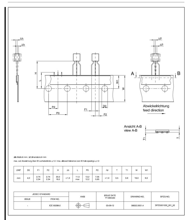
Fig. 3–5: TO92U-1: Dimensions ammopack inline, spread
