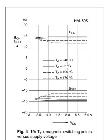
**Note:** In the diagram "Magnetic switching points versus ambient temperature" the curves for  $B_{ON}$ min,  $B_{ON}$ max,  $B_{OFF}$ min, and  $B_{OFF}$ max refer to junction temperature, whereas typical curves refer to ambient temperature.
