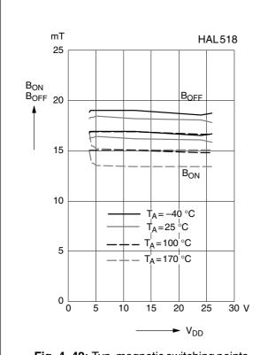
**Fig. 4–42:** Typ. magnetic switching points versus supply voltage
