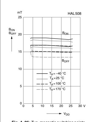
**Fig. 4–26:** Typ. magnetic switching points versus supply voltage
