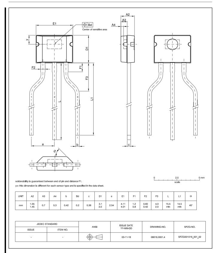
**Fig. 3–2: TO92UA-1**: Plastic Transistor Standard UA package, 3 leads, spread Weight approximately 0.105 g
