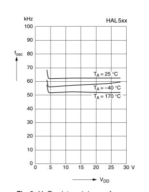
**Fig. 3–11:** Typ. Internal chopper frequency versus supply voltage
