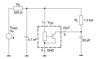
Fig. 5-1: Test circuit for EMC investigations
