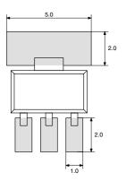
**Fig. 3–6:** Recommended pad size SOT89B-1 Dimensions in mm
