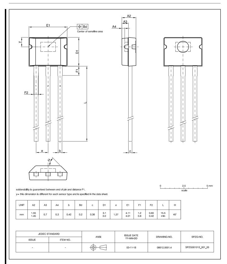
**Fig. 3–3: TO92UA-2**: Plastic Transistor Standard UA package, 3 leads Weight approximately 0.105 g
