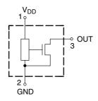
Fig. 1-1: Pin configuration
