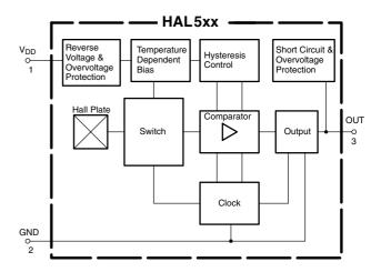
Fig. 2-1: HAL5xx block diagram
