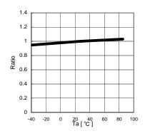
Fig.8 IOUT Temperature dependency ( 100 lx )
