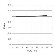
Fig.9 IOUT VCC dependency
