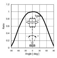
Fig.4 Directional Characteristics 1
