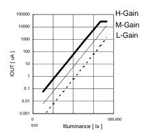
Fig.3 Illuminance – IOUT Characteristics
