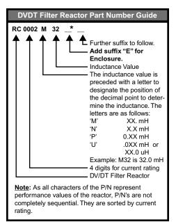
Add the Suffix "E" to the standard part number below for an Enclosed unit.
