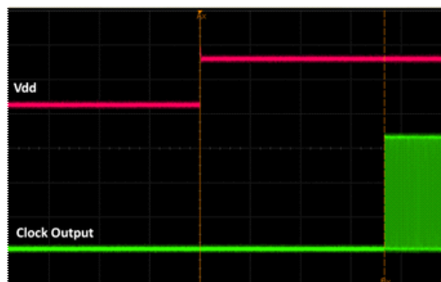
Figure 17. Startup Waveform vs. Vdd
