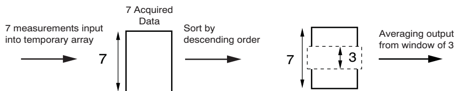
Figure 28. MAV Filter Operation (Patent Pending)
