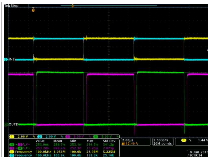
Figure 38. Bench Test Waveform for INA/B and OUTA/B
