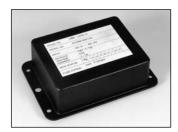
The MBR series consists of low power encapsulated converters which incorporate full surge and transient protection to RIA12 and EN50155. They are available in single, dual, and triple output versions, with nominal inputs from 24V up to 110V. Normally supplied with pins for PCB mounting, they are also available with flying leads for bulkhead mounting.
