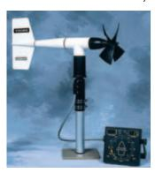
For offshore and marine use, **Model 05106**, **Wind Monitor-MA** features special waterproof bearing lubricant and a sealed, heavy duty cable pigtail in place of the standard junction box. Separate signal conditioning for voltage or current outputs is available.
