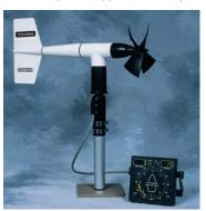
Wind Sensor Interface offers calibrated 0-5VDC outputs for wind speed and wind direction. Model 05631C Wind Line Driver provides calibrated 4-20 mA current signals for each channel, useful in high noise areas or for long cables of up to several kilometers. Each interface circuit is supplied in a weatherproof junction box with mounting hardware for installation near the sensor.
