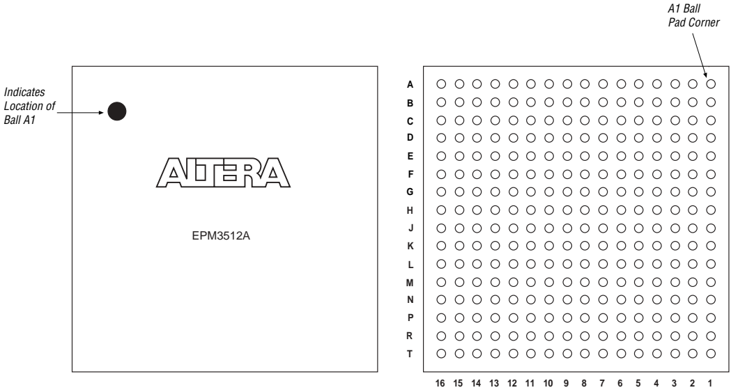
Figure 18. 256-Pin FineLine BGA Package Pin-Out Diagram
