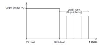
Additionally, if the  $I_{\rm O}$  is <250% but >110% for a prolong period of time (depending on the load), the Over Temperature Protection (OTP) will be activated due to high temperature on critical components. The power supply will then go into hiccup mode until the fault is removed; and, the input voltage is removed, then reapplied.
