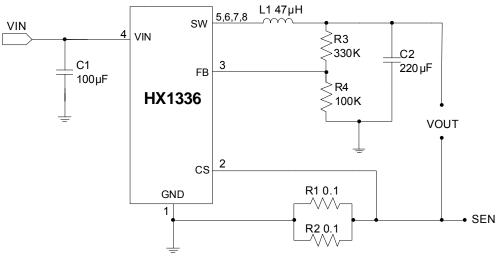
\*The output voltage is set by R3 and R4:  $V_{OUT} = 1.21V \cdot [1 + (R3/R4)]$ .
