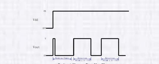
Cautions) Warm-up Time: Max. 30 sec. Regarding of detection or non-detection during the waiting time, ON signal may be made due to Instability of circuit
