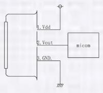
Fig.4:Basic Application Circuit Examples
