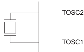
Figure 7-3. Crystal Oscillator Connections
