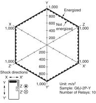
Conditions: Shock is applied in  $\pm X$ ,  $\pm Y$ , and  $\pm Z$  directions three times each with and without energizing the Relays to check the number of contact malfunctions.
