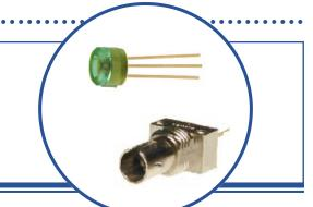
The OPF520 series fiber optic receiver is a high performance device packaged for data communications links. As such, it is designed to work with fiber core diameters from 50µm to 200µm and over a broad input power range. The construction contains a monolithic photo-IC comprised of a photodiode, biasing network, DC amplifier and an open collector output transistor. The output circuitry makes this device compatible with TTL and CMOS logic.
