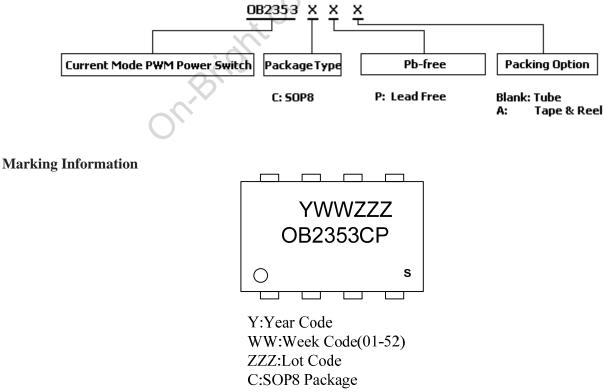
C:SOP8 Package P:Pb-free Package S:Internal Code(Optional)
