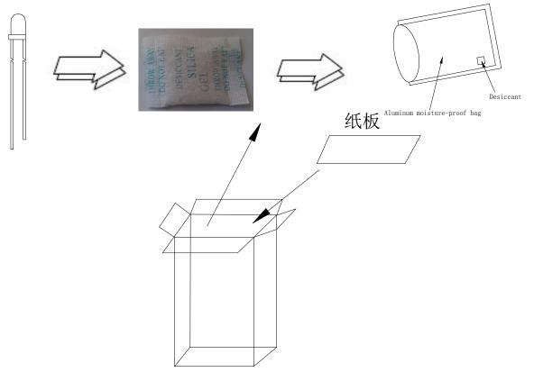
The packing way: Electrostatic bag packing
