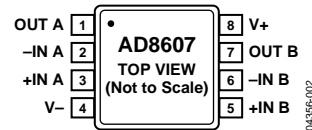
Figure 2. 8-Lead MSOP (RM Suffix)
