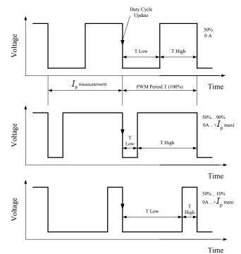
$$PWM \ period \ T_{Period} = T_{High} + T_{Low}$$
