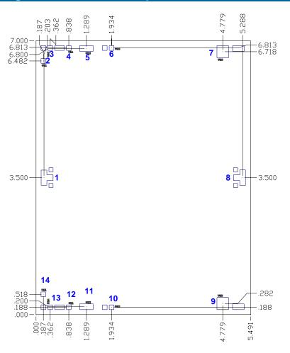
Unit: millimeters Thickness: 0.10 Die x, y size tolerance: +/- 0.050 Chip edge to bond pad dimensions are shown to center of pad Ground is backside of die
