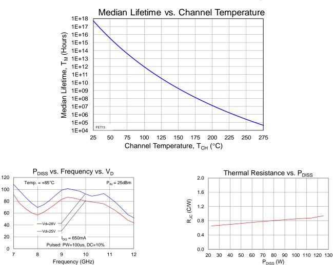
Test Conditions:  $V_D = 40$  V; Failure Criteria = 10% reduction in  $I_{D_MAX}$
