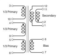
Primary windings to be connected in series on the PC board. Secondary winding to be connected in parallel on the PC board.
