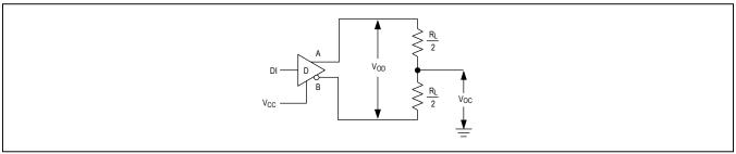
Figure 1. Driver V<sub>OD</sub> and V<sub>OC</sub>
