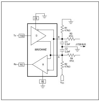
Figure 15. J1708 Application Circuit
