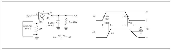
Figure 5. Driver Enable and Disable Times
