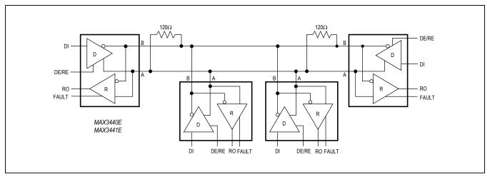
Figure 13. MAX3440E/MAX3441E Typical RS-485 Network
