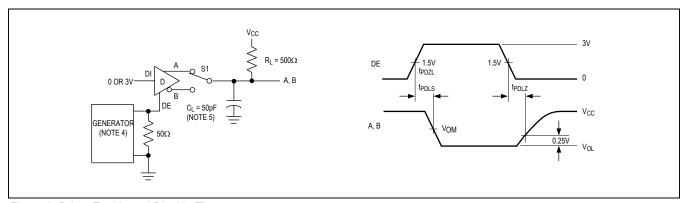
Figure 6. Driver Enable and Disable Times
