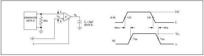
Figure 7. Receiver Propagation Delay
