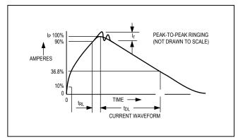
Figure 9b. Human Body Model Current Waveform
