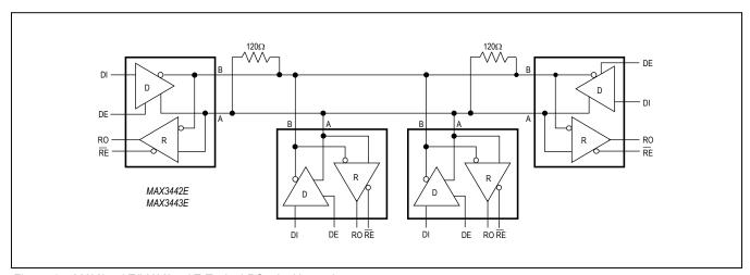
Figure 14. MAX3442E/MAX3443E Typical RS-485 Network
