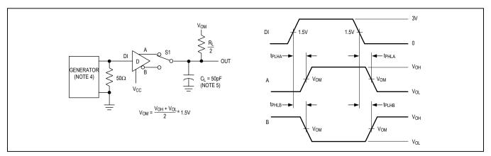
Figure 3. Driver Propagation Times
