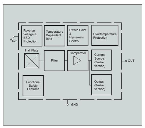
Fig. 1: Block diagram of the HAL 15xy
