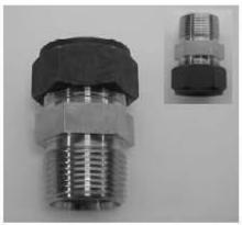
Metal Process Connector PN 23166-xx (xx - 00 for 316 SST and xx = 01 for titanium) can be used for insertion or submersion Model 396 sensor connection to 1-inch tee fittings. It also must be used to connect Model 396R to ball valve PN 23240-00 or directly to the process.
