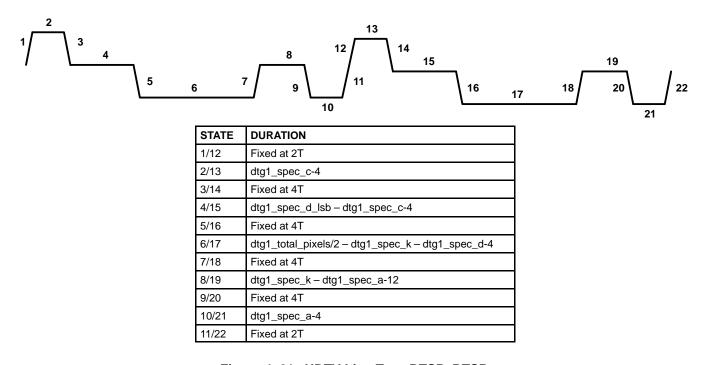
Figure 4–21. HDTV Line Type BTSP\_BTSP
