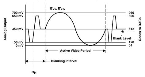
Figure 4–46. Analog Output of Cr and Cb Channels With Sync Insertion
