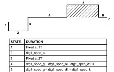
Figure 4-35. SDTV Line Type NSP\_ACTIVE
