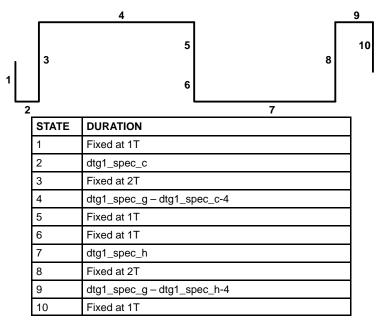
Figure 4-32. SDTV Line Type NEQ\_BSP
