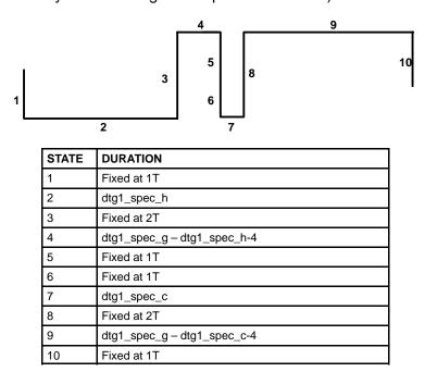
Figure 4-33. SDTV Line Type BSP\_NEQ
