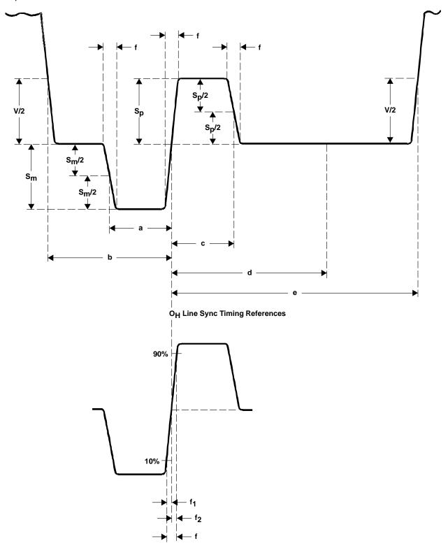
Figure 4–16. Tri-Level Line-Synchronizing Signal Waveform
