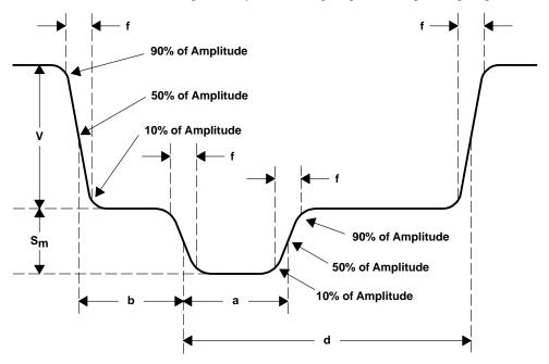
Figure 4–26. Horizontal Synchronization Signal Waveform
