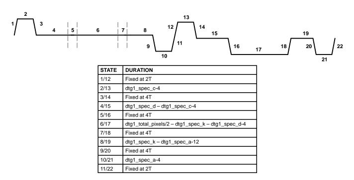
Figure 4-22. HDTV Line Type NTSP\_BTSP
