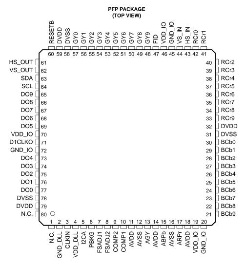
Figure 2–1. THS8200 Pin Location Diagram
