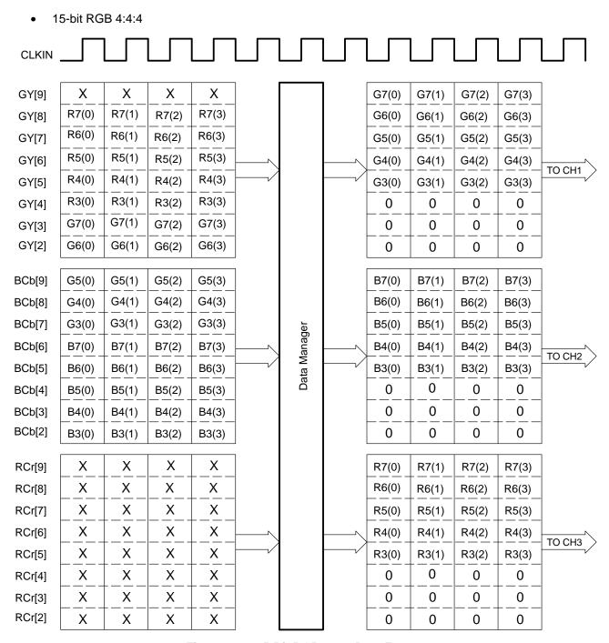
Figure 4-4. 15-Bit RGB 4:4:4 Data Format
