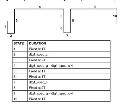
Figure 4–28. SDTV Line Type NEQ\_NEQ
