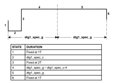
Figure 4-34. SDTV Line Type FULL\_NEQ
