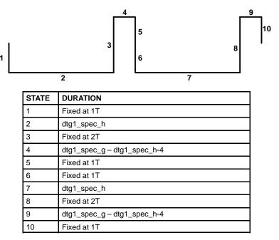
Figure 4-30. SDTV Line Type BSP\_BSP
