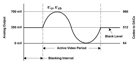
Figure 4-45. Analog Output of Cr and Cb Channels Without Sync Insertion
