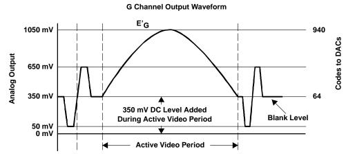
Figure 4-41. G-Channel Output Waveform
