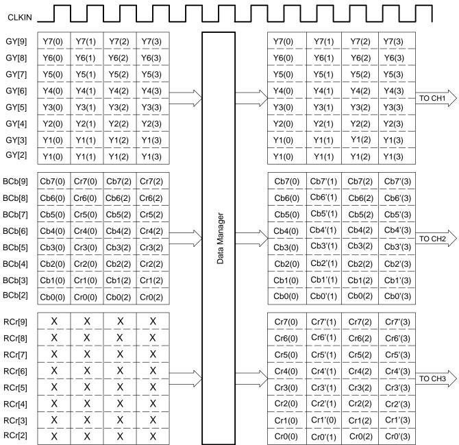
NOTE: Where Cb'Cr' are the output of half-band interpolation filter.
