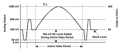
Figure 4-44. Y-Channel Output Waveform
