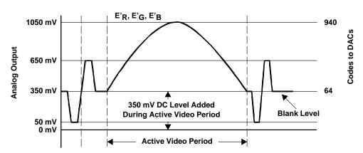
Figure 4-43. R-, G-, and B-Channel Output Waveform
