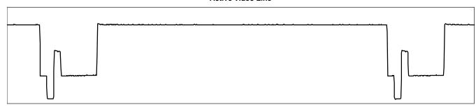
Figure 7–1. THS8200 Output Waveforms for 1080I: Vertical Blanking in First and Second Fields, and Active Video
