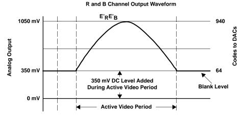
Figure 4-42. R- and B-Channel Output Waveform
