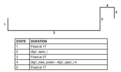
Figure 4-29. SDTV Line Type FULL\_BSP
