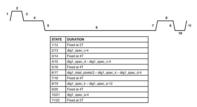
Figure 4-24. HDTV Line Type FULL\_BTSP
