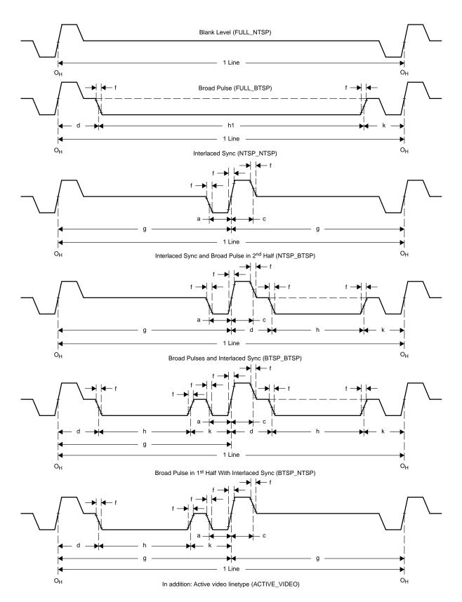
Figure 4-17. THS8200 VBI Line Types in HDTV Mode
