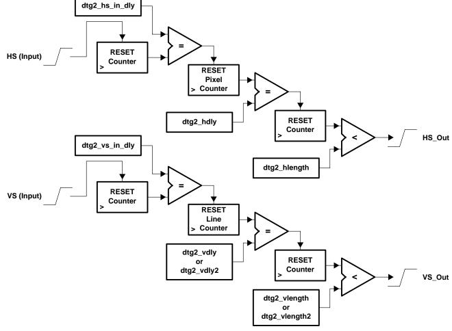
Figure 4-15. THS8200 DTG VS/HS Output Generation
