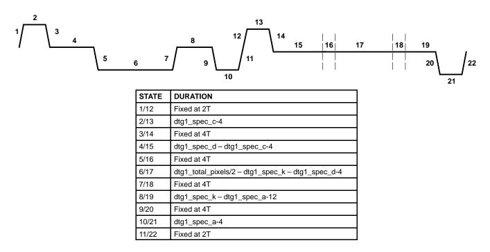
Figure 4–23. HDTV Line Type BTSP\_NTSP
