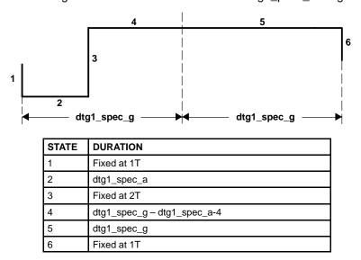
Figure 4-31. SDTV Line Type FULL\_NSP
