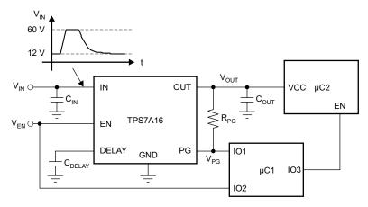
Figure 18. Low-Power Microcontroller Rail Sequencing in Automotive Applications Subjected to Load-Dump Transients
