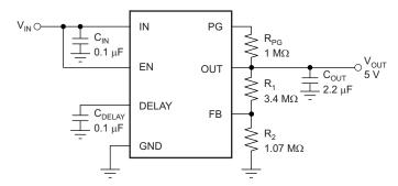
Figure 15. Adjustable Operation
