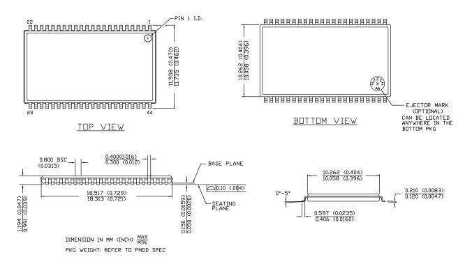
Figure 10. 44-pin TSOP Z44-II Package Outline, 51-85087
