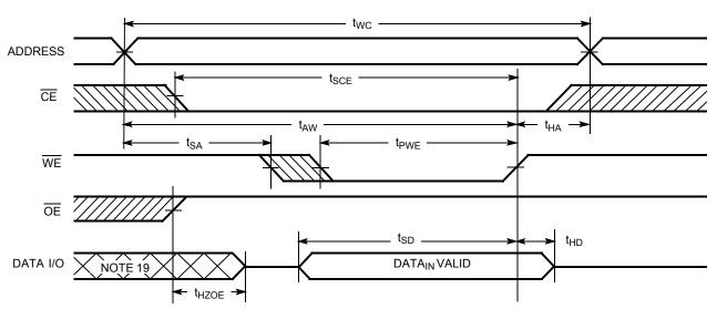
Figure 7. Write Cycle No. 1 (WE Controlled, OE HIGH During Write) <sup>[17, 18]</sup>
