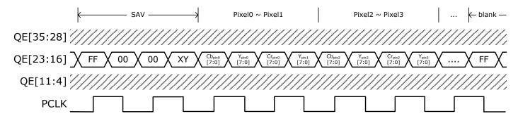
Figure 12. 8-bit CCIR-656 dual-edges triggered with 0.5X PCLK
