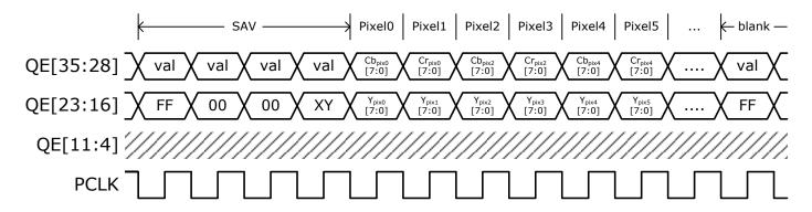
Figure 9. 16-bit YCbCr 4:2:2 with embedded syncs
