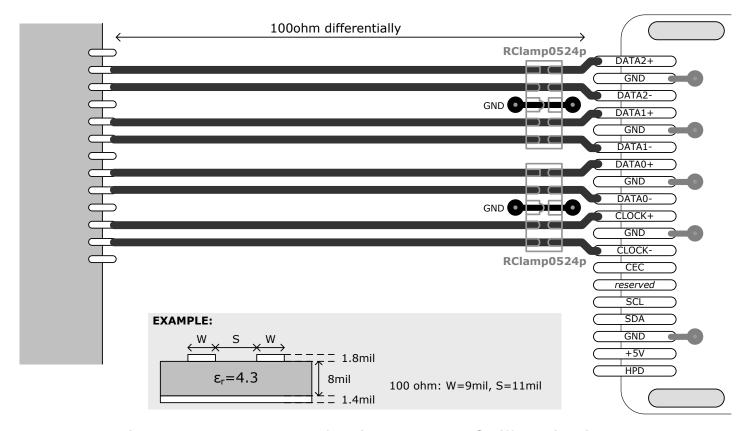
Figure 18. Layout example for high-speed TMDS differential signals
