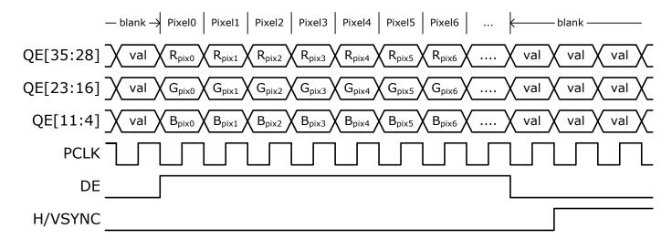
Figure 5. 24-bit RGB 4:4:4 Timing Diagram
