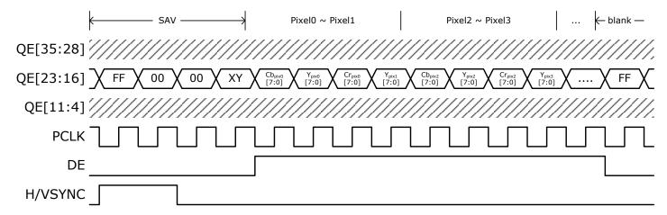
Figure 13. 8-bit CCIR-656 + separate syncs
