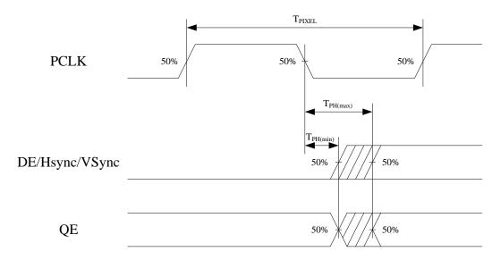
Figure 4. PCLK falling edge to transition time under single-pixel mode
