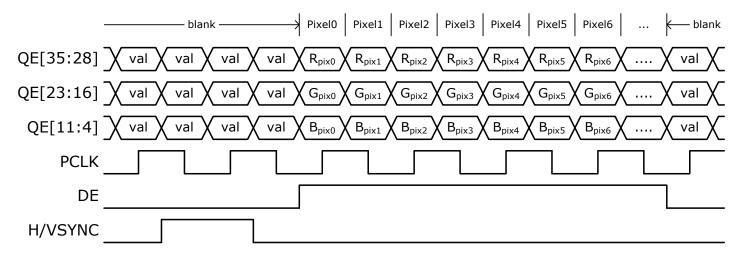
Figure 6. 24-bit RGB 4:4:4 dual-edges triggered with 0.5X PCLK
