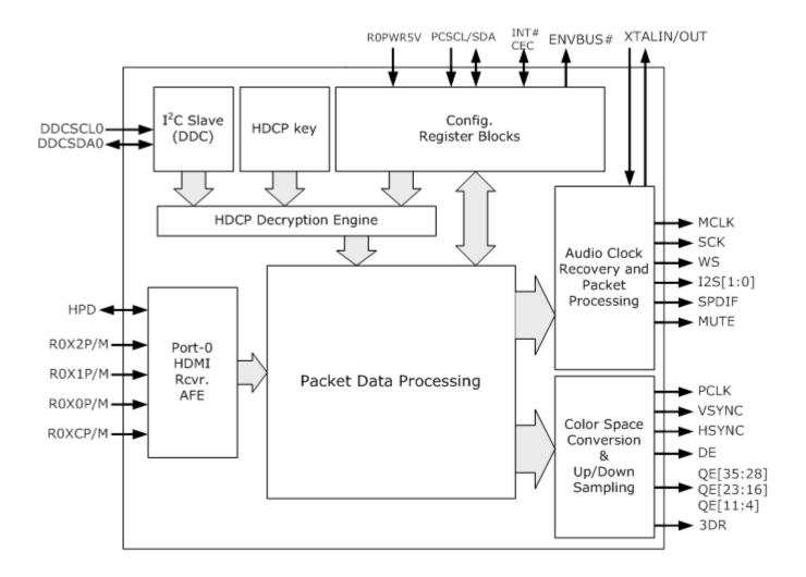
Figure 2. Functional block diagram of the IT66021FN
