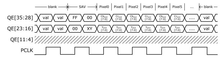
Figure 16. 16-bit BTA1004 dual-edges triggered with 0.5X PCLK
