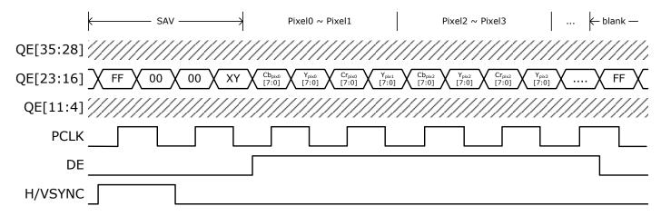
Figure 14. 8-bit CCIR-656 + separate syncs dual-edges triggered with 0.5X PCLK
