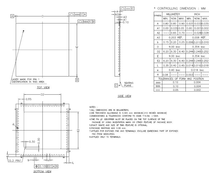
Figure 19. 76-pin QFN Package Dimensions
