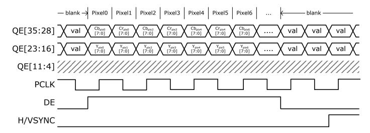
Figure 8. 16-bit YCbCr 4:2:2 with separate syncs dual-edges triggered with 0.5X PCLK
