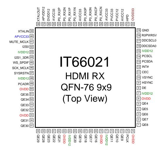
Figure 1. IT66021FN pin diagram
