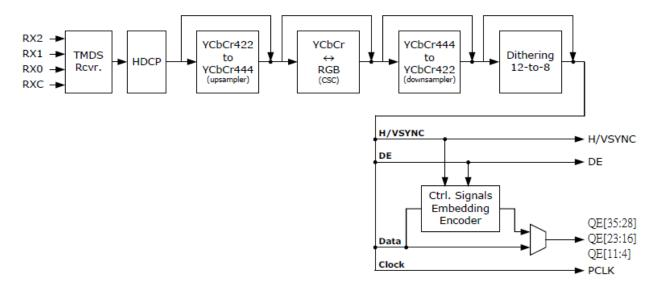
Figure 3. Video Data Processing flow of the IT66021FN
