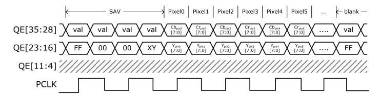
Figure 10. 16-bit YCbCr 4:2:2 with embedded syncs dual-edges triggered with 0.5X PCLK
