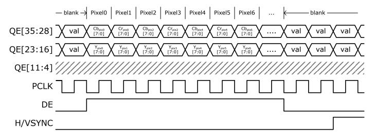
Figure 7. 16-bit YCbCr 4:2:2 with separate syncs
