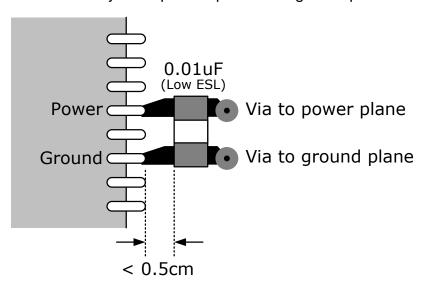
Figure 17. Layout example for decoupling capacitors.
