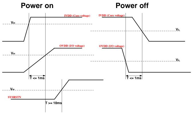
When power on, please keep IVDD go VIH before OVDD go VIH (IVDD must supply earlier than or equal to OVDD). And please keep the time interval between IVDD and OVDD shorter than 1ms when power on or power off.
