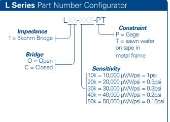
**Example:** L10-20K-PT offers 5kohm Impedance, Open Bridge, 20,000 µV/V/psi and Gage Constraint
