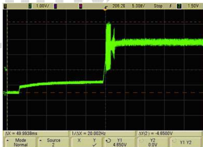
Figure 8. Input Voltage Overshoot >4V (Bad)
