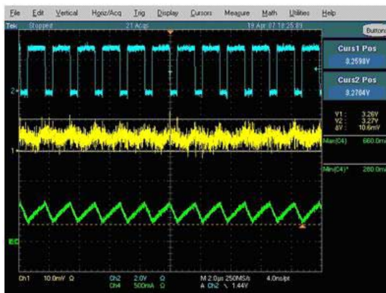
Figure 9. Ceramic 22µF 1210(X5R) (Good)
