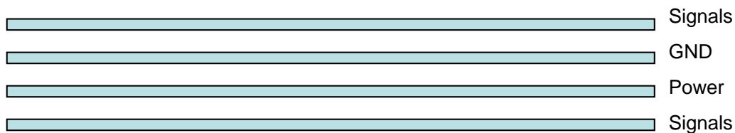
Figure 29: Typical 4-layer PCB construction
