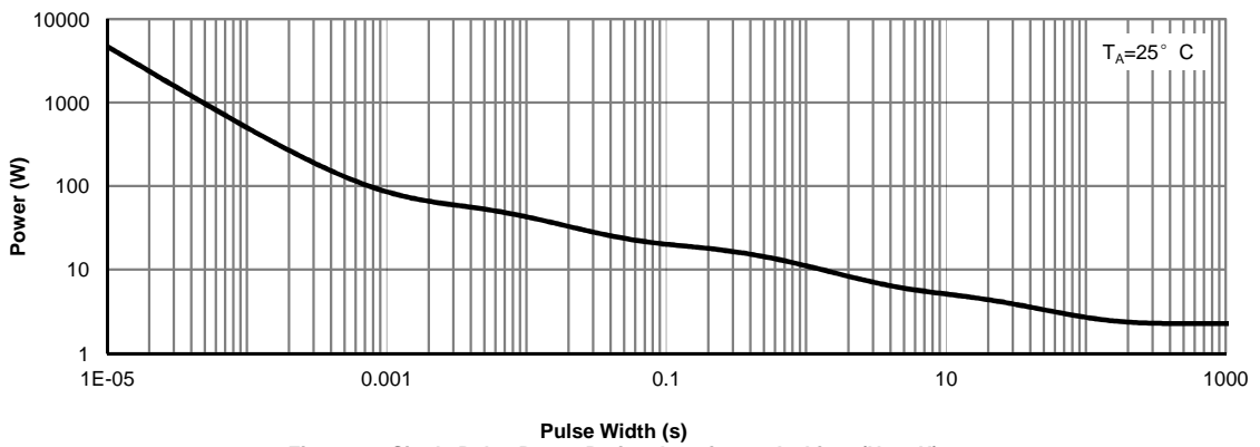
Figure 14: Single Pulse Power Rating Junction-to-Ambient (Note H)
