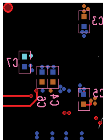
Figure 63. Bottom Layer Decoupling
