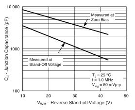
Fig. 4 - Typical Junction Capacitance
