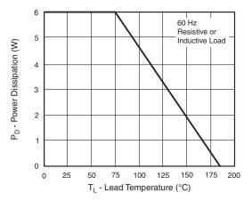
Fig. 6 - Power Derating Curve
