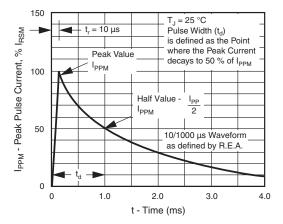
Fig. 3 - Pulse Waveform
