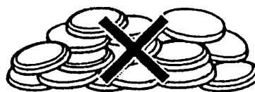
Example of stacked and jumbled batteries
