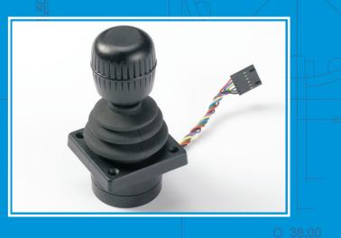
CLASS LEADING INSTALLED DEPTH <19 MM - HALL EFFECT SENSING ONE, TWO OR THREE AXES - 5V OR 3.3V OPERATION EMC SHIELDED - ANALOGUE OR PWM OUTPUTS NEXT GENERATION METAL MECHANISMS
