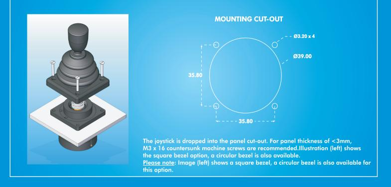
Note: The dimensions shown are for a generic 3000 Series with the E type handle. For specific dimensions of this or any other configuration please refer to Apem.
