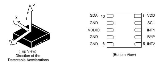
Figure 2. Direction of the detectable accelerations
