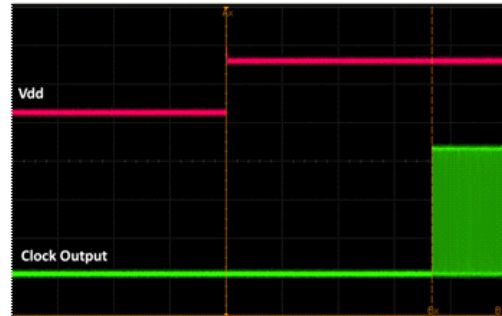
Figure 17. Startup Waveform vs. Vdd
