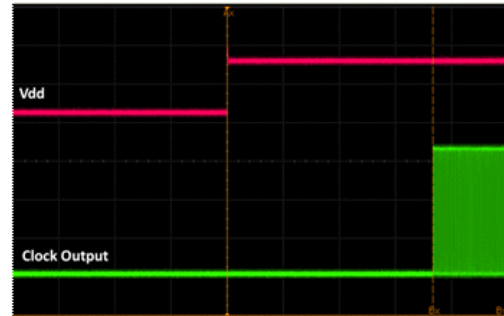
Figure 16. Startup Waveform vs. Vdd
