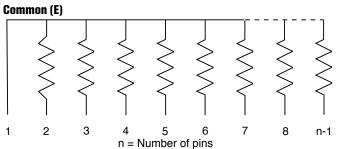
Common parts are characterised by having a number of resistive elements, all of the same nominal value. All elements are connected to pin 1.
