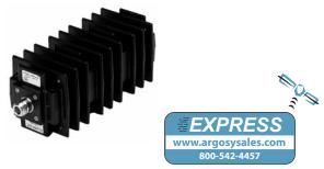
POWER RATING: 250 watts average (mounted horizontally assuming unobstructed air flow and natural convection around unit) @ 25°C ambient temperature, derated linearly to 25 watts @ 125°C. 10 kilowatts peak
