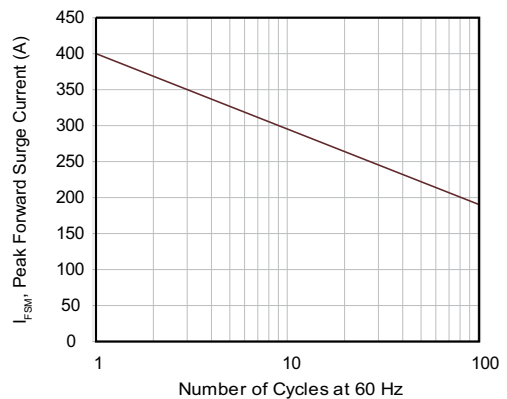
Figure 6 - Maximum Non-Repetitive Forward Surge Current Uni-Directional Only
