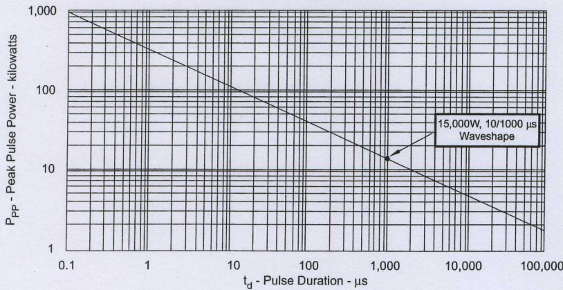
FIGURE 1 PEAK PULSE POWER VS PULSE TIME
