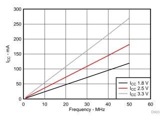
Figure 5. I<sub>CC</sub> vs Frequency
