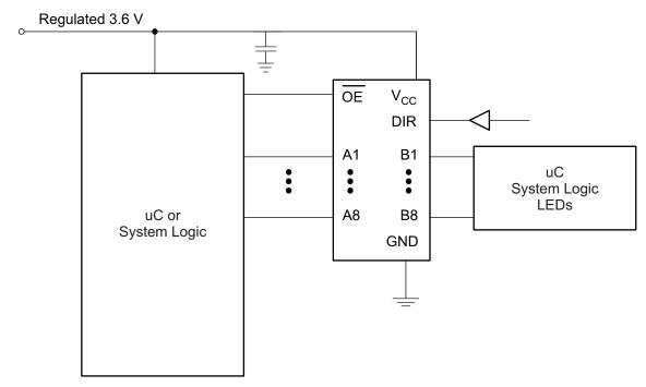
Figure 4. Typical Application Schematic
