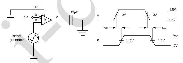
Figure 5A. test circuit
