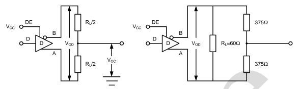
Figure 1A. V<sub>OD</sub> and V<sub>OC</sub>
