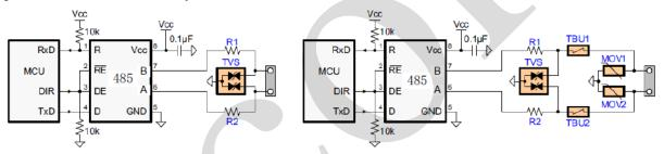
Figure 10. Transient Protections Against ESD, EFT, and Surge Transients
