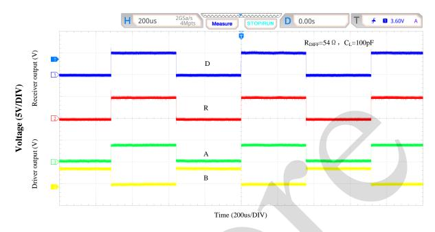
Figure 7. driver and receiver waveforms
