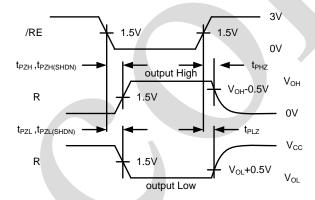
Figure 6B. measurement points Figure 6. receiver enable and disable times
