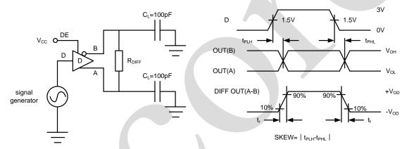
Figure 2A. test circuit
