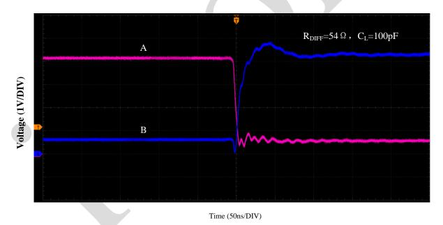
Figure 8. driver waveforms
