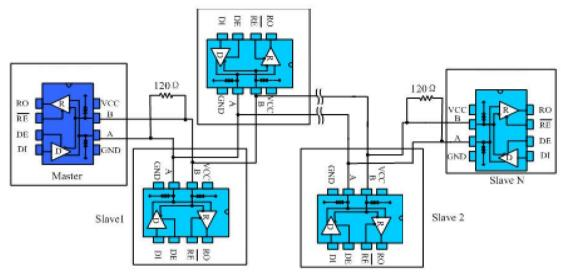
Fig. 10 Hand-in-hand type RS485 half-duplex communication network
