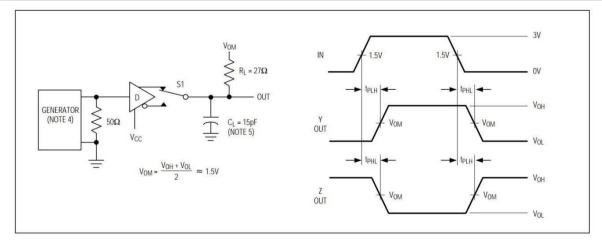
Fig. 4 Driver propagation times
