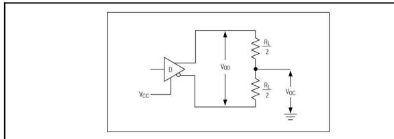
Fig. 2 Driver DC test load
