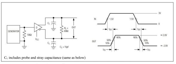
Fig. 3 Driver differential output delay and transition times
