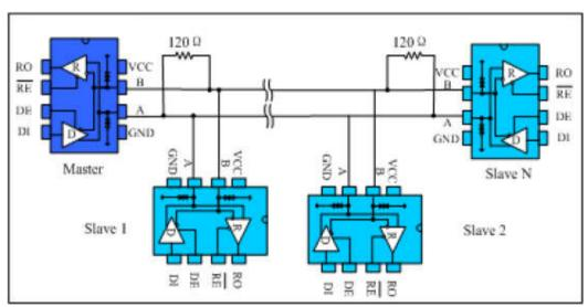
Fig. 9 Bus-type RS485 half-duplex communication network
