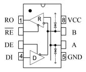
Figure 1 MAX3485E pin configuration
