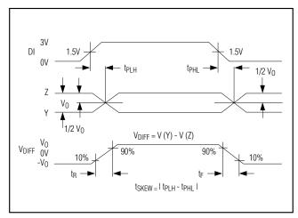
Figure 5. Driver Propagation Delays
