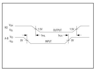
Figure 7. Receiver Propagation Delays
