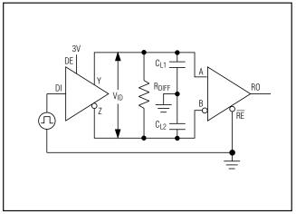
Figure 3. Driver/Receiver Timing Test Circuit
