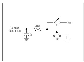
Figure 4. Driver Timing Test Load
