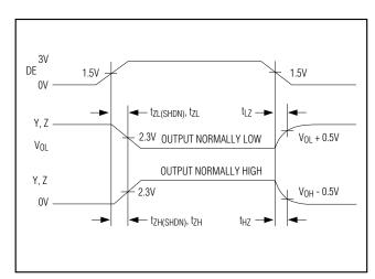
Figure 6. Driver Enable and Disable Times
