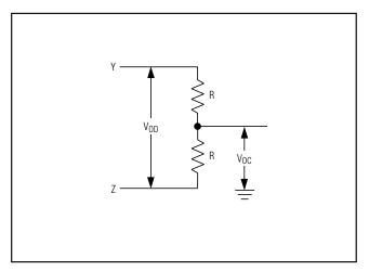
Figure 1. Driver DC Test Load
