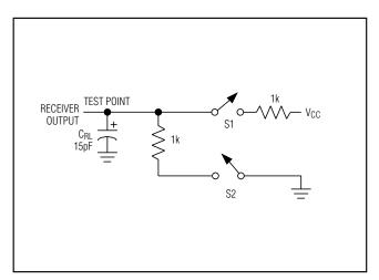
Figure 2. Receiver Timing Test Load
