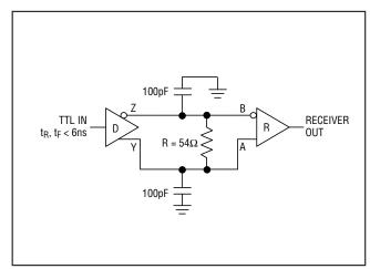
Figure 10. Receiver Propagation-Delay Test Circuit
