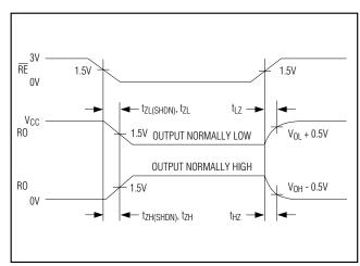
Figure 8. Receiver Enable and Disable Times
