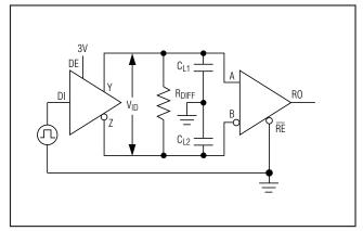
Figure 6. Driver/Receiver Timing Test Circuit
