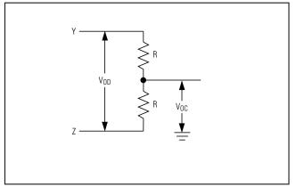
Figure 4. Driver DC Test Load
