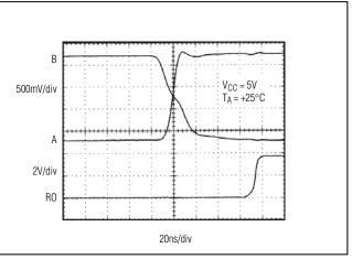
Figure 16. MAX481/MAX485/MAX490/MAX491/MAX1487 Receiver t<sub>PLH</sub>
