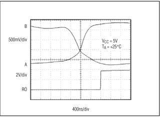
Figure 18. MAX483, MAX487–MAX489 Receiver tPLH
