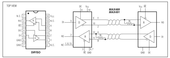
Figure 3. MAX489/MAX491 Pin Configuration and Typical Operating Circuit
