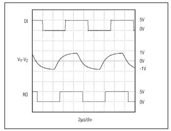
Figure 19. MAX481/MAX485/MAX490/MAX491/MAX1487 System Differential Voltage at 110kHz Driving 4000ft of Cable Figures 21 and 22 show typical network applications circuits. These parts can also be used as line repeaters, with cable lengths longer than 4000 feet, as shown in Figure 23.
