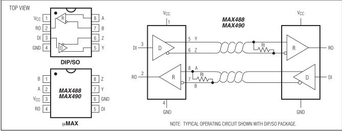
Figure 2. MAX488/MAX490 Pin Configuration and Typical Operating Circuit
