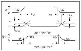
Figure 8. Driver Propagation Delays
