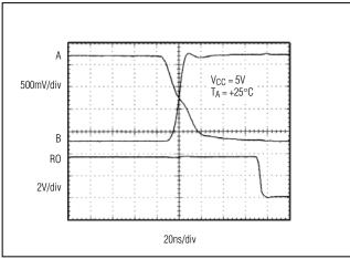
Figure 15. MAX481/MAX485/MAX490/MAX491/MAX1487 Receiver t<sub>PHL</sub>
