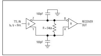
Figure 14. Receiver Propagation Delay Test Circuit
