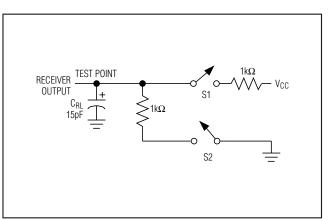
Figure 5. Receiver Timing Test Load
