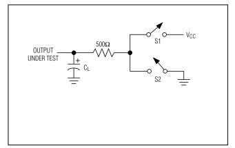
Figure 7. Driver Timing Test Load
