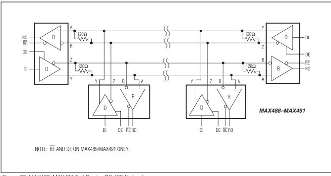
Figure 22. MAX488–MAX491 Full-Duplex RS-485 Network
